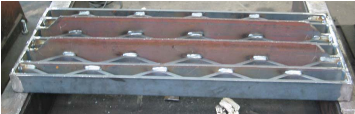
Figure 3 – Underside of modified flat grate
