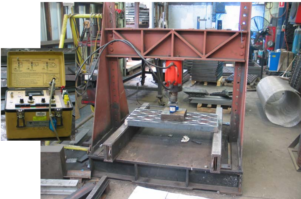
Figure 2 – Testing rig with flat grate
